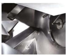
Mixing flights produce a tumble-turn-cut-fold mixing action that yields batch uniformity in less than three minutes.
