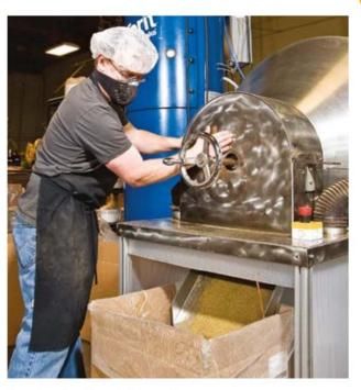
The mixer is self emptying resulting in total discharge and no waste.
